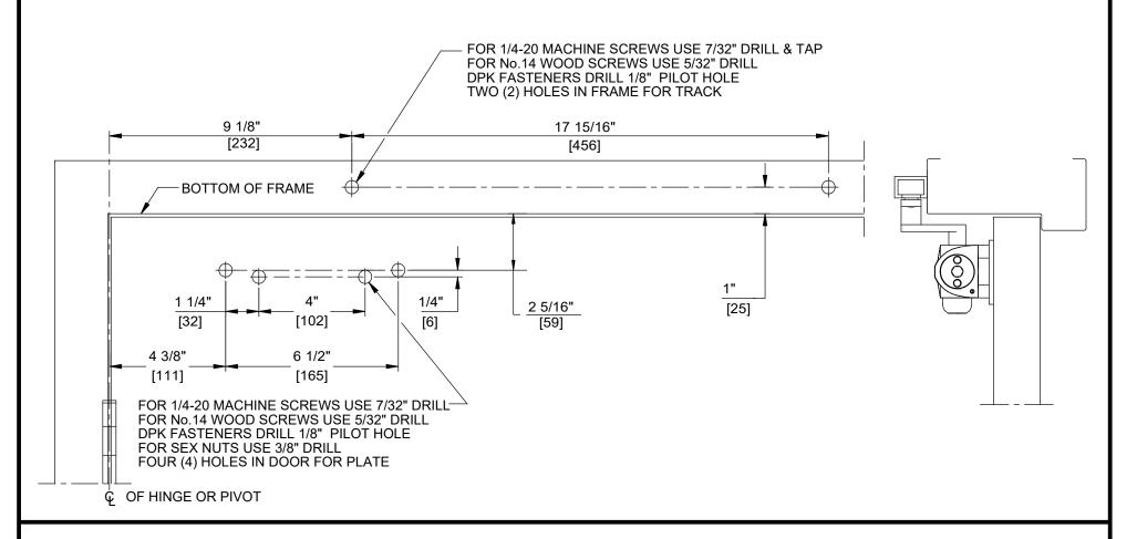
DOOR CLOSER MODELS: 7414, 7436 TDE, TDEH DOUBLE EGRESS TRACK INSTALLATION (PULL SIDE MOUNT) WITH PLATES BP74, BP86, BP86FC
